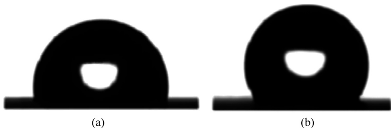
Figure 4. Micrograph of static contact angle: (a) electrospun at 10 KV, (b) electrospun at 22 KV.
